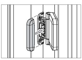
To fasten the cover to the hinge, screw in the set screw (see illustration) completely by turning it clockwise with a hexagon spanner.
