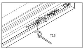
Adjusting the gasket pressure at the side of the sash at the top.
