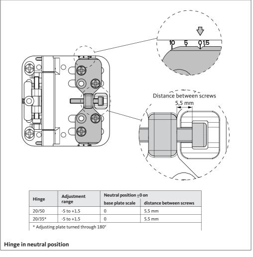
You can adjust the vertical position of the Fold&Slide sashes relative to one another and also the shadow gap between the sashes when installed by turning the set screws at the hinge (see figure "Adjustment of the hinge" on page 5):
