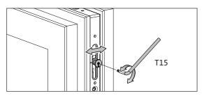
Adjusting the gasket pressure at other locking points on the underside of the sash.
