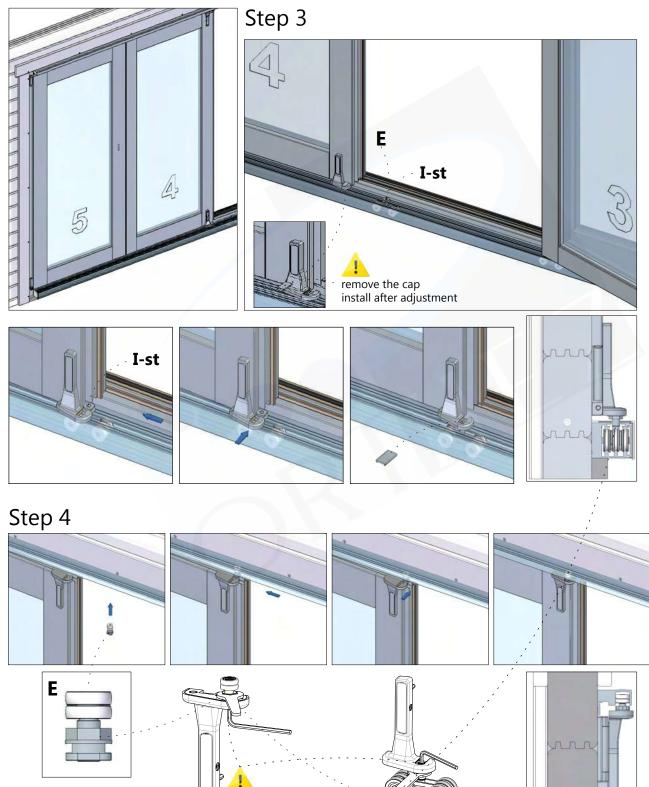
□ remove the cap □ install after adjustment
