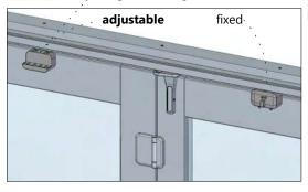
□ loosen bolts to adjust **up and down** □ tighten bolts after adjustment
